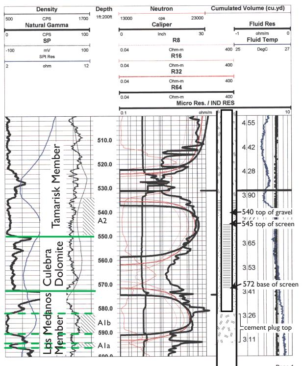
Preliminary Selection of Screened Interval, Cement Plug, Page 1 and Gravel Pack Interval for SNL-9
