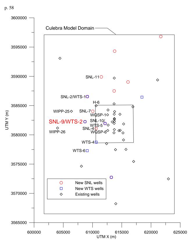
Figure 18. Pumping well and principal observation wells for western multipad pumping test.
